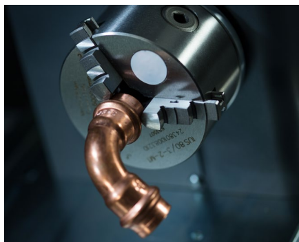
Rotary accessory for cylindrical parts marking
