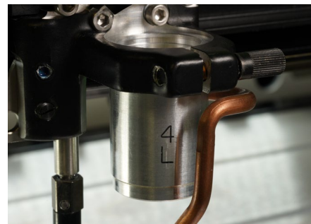
Lens 4.0" Thick cutting and fast engraving
